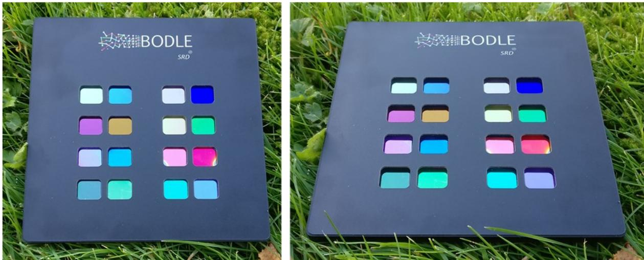
**Figure 3** – Various colours obtained by tuning the thickness of the PCM based, thin-film stack. Each stack is shown in both the amorphous and crystalline phase. The same collection of stacks is photographed at two different angles to demonstrated the low angle dependence obtainable by the technology.
